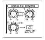
Fig. 2.9: Stereo aux return controls
